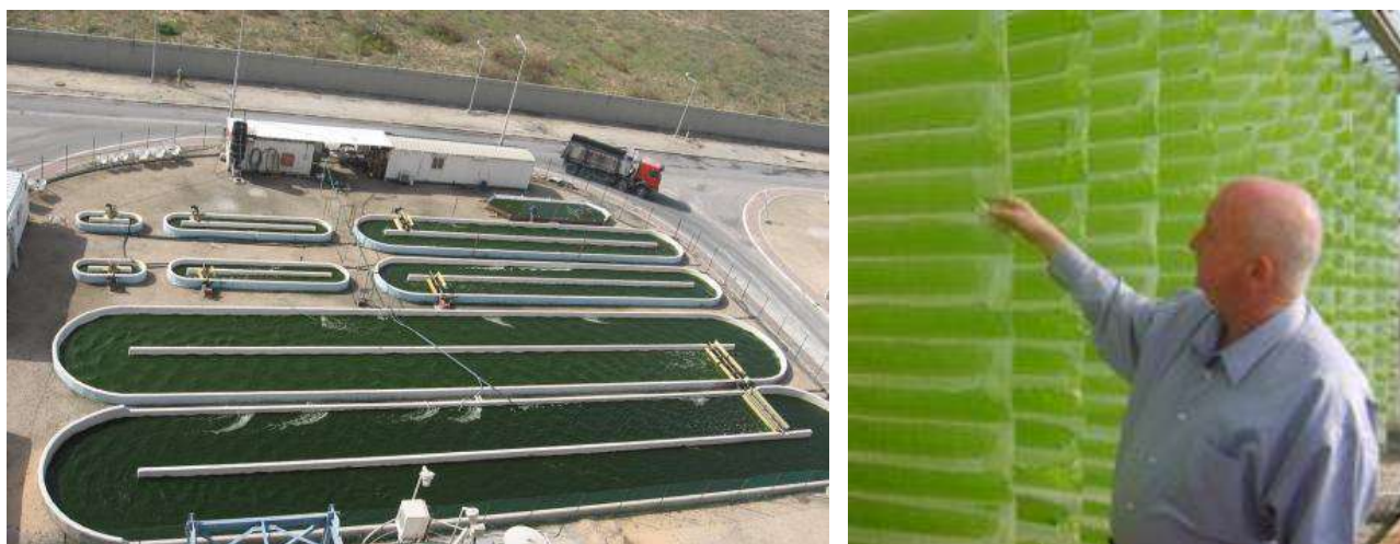
Figure 9.8. Pilot microscopic algae farms. Sources: Left: artificial open lake systems, < http://www.makebiofuel.co.uk/biofuel-from-algae >. Right: photobioreactor system, < http://www.enn.com/energy/article/37961 >.
