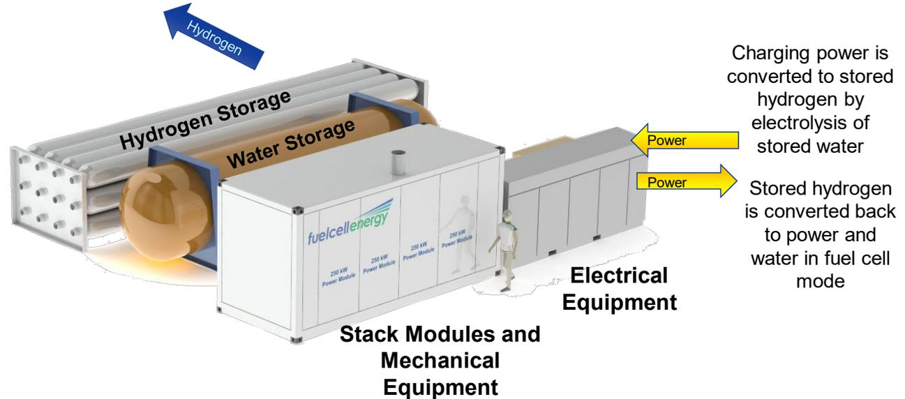
Charging power is converted to stored hydrogen by electrolysis of stored water
