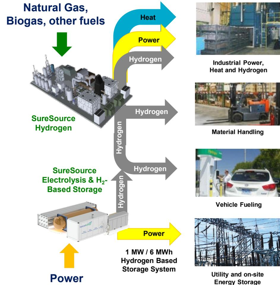
**Broad portfolio of hydrogen technologies based on carbonate and solid oxide platforms**
