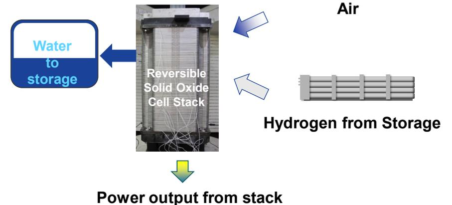
With water as the only stored reactant, hydrogen based storage has significant advantages for long duration
